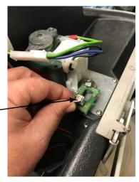
6. Remove the mixingmotor assebly by removing the 4 screws holding it on place
