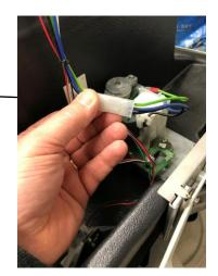
5. Disconect the connector in the PCB card on the motor.
