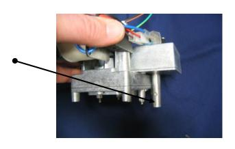
9. Remove the rest of the old shear pin, use a hammer and make sure that the axle have a solid ground when you work.
