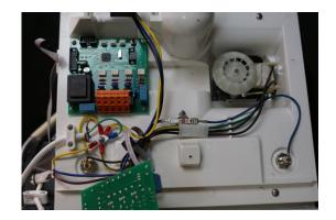
Then disconnect the cables in pairs, one in the upper and one in the lower row in the terminal on the old card. Move to the new circuit board, to the same place.
