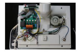
Remove all connection cables from the old pcb
