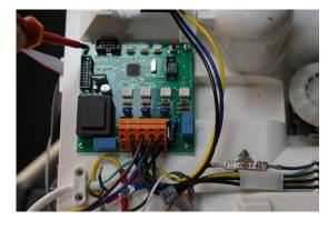
Put the new card in place with the 4 screws. Install the blue and brown cable in the upper and lower rows on the far left of the terminal block.
